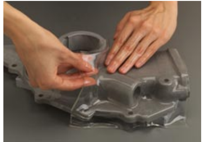
Figure 1. PhotoStress coating being contoured to the surface of a vehicle water pump casting.
